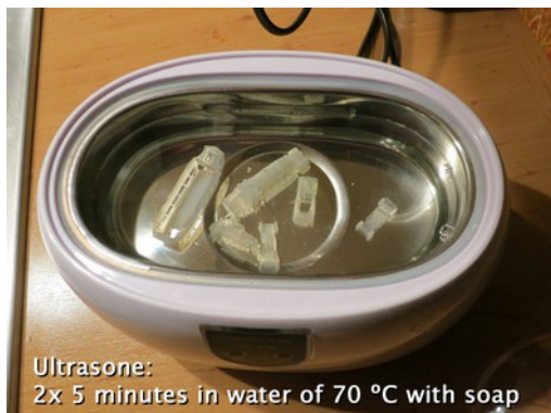
Acetone: Max 5 minutes! Clean afterwards with water (with ultrasone)
