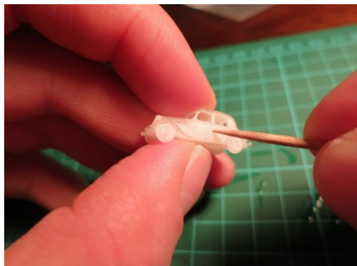
Ultrasonie: 2x 5 minutes in water of 70 °C with soap
