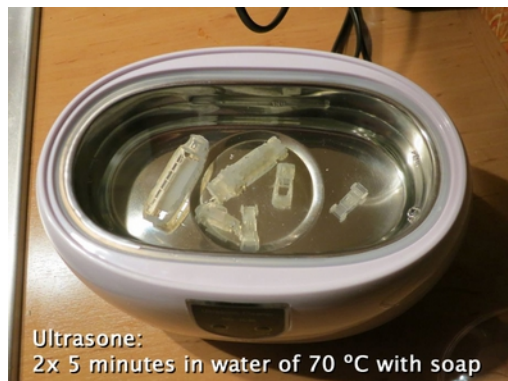
Acetone: Max 5 minutes! Clean afterwards with water (with ultrasonie)
